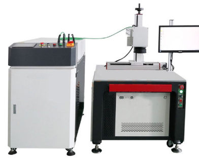
Fig. 3. Experimental system for laser welding.
